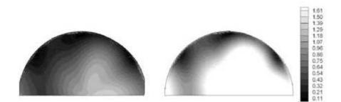
Fig. 1. Stress intensity of the ball.
