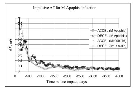
Fig. 1. Impulsive  $\Delta V$  required to successfully deflect the fictitious asteroid M-Apophis and cause it to miss Earth's surface by 3 Earth radii. There is virtually no difference in the  $\Delta V$  requirements for accelerating or decelerating the asteroid.
