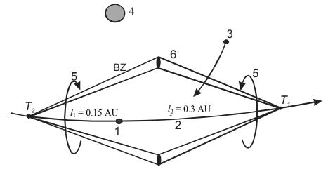
Fig. 1. The cut of the closed barrier zone by the ecliptic plane: l — the Earth; 2 — the Earth orbit; 3 — small body; 4 — the Sun; 5 — survey scans of near-Earth space with (6) rotating fields of view of the space telescopes  $T_1$ and  $T_2$  (barrier zone).
