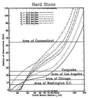
Fig. 2. Area of destruction versus impactor size and velocity, from Hills and Goda [11].
