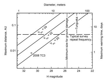
Fig. 6. Short-term warning provided by an optical survey.
