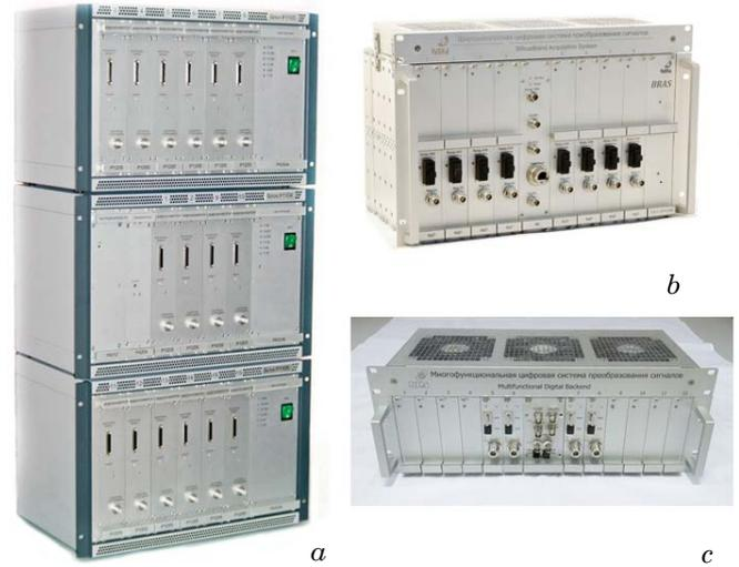
Fig. 2. Digital data acquisition systems developed in IAA RAS in the last ten years. *a* – R1002M DAS; *b* – Broadband Acquisition System; *c* – Multifunctional Digital Backend with 4 channels inserted
