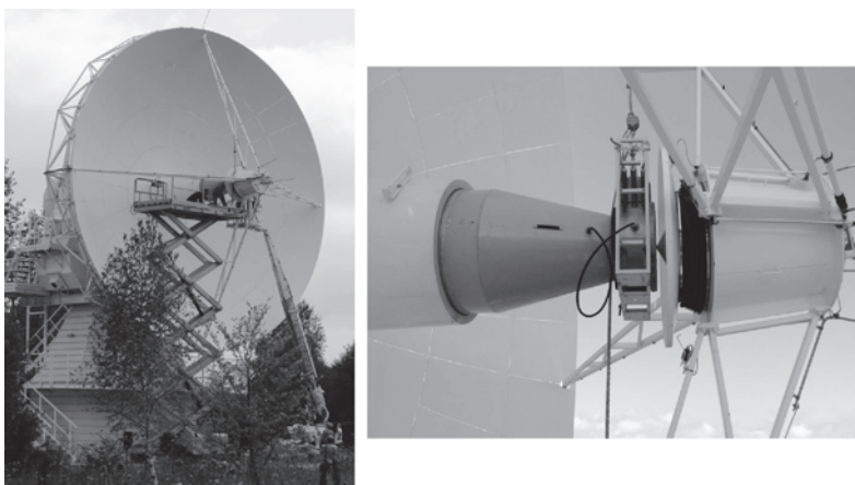
Fig. 1. The RT-13 noise temperature measurements by using wide-aperture low-temperature noise generator
