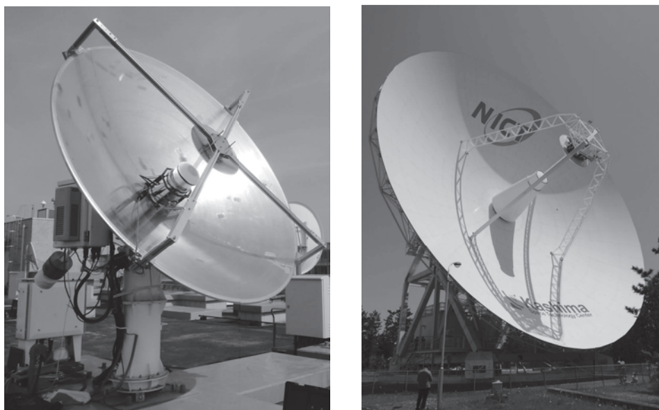
Fig. 1. Broadband compact antenna No. 2 (MARBLE 2) in Tokyo ( left ) and Kashima 34 meter in Ibaraki ( right )
