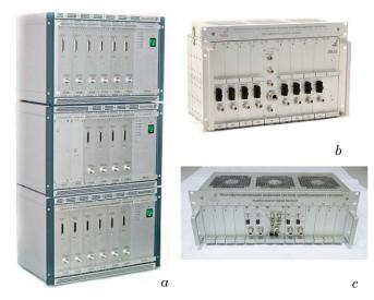
Fig. 2. Digital data acquisition systems developed in IAA RAS in the last ten years. a - R1002M DAS; b - Broadband Acquisition System; c - Multifunctional Digital Backend with 4 channels inserted
