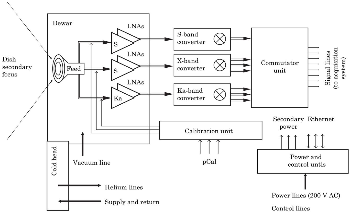
Fig. 1. Schematic diagram of the tri-band receiver focal module
