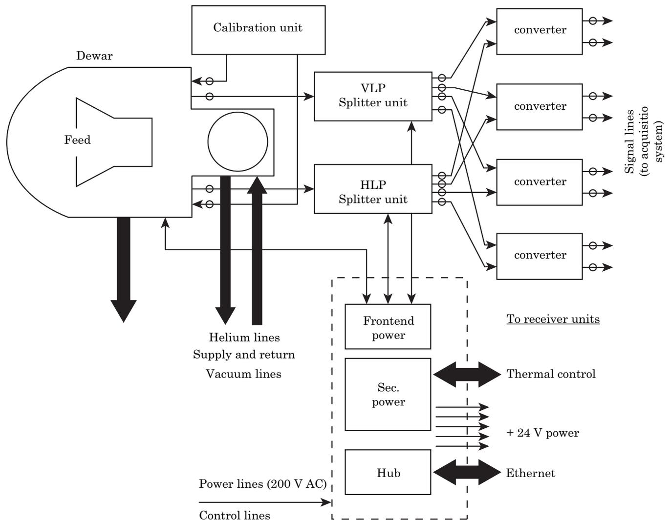
Fig. 2. Schemantic diagram of the wideband receiver focal module
