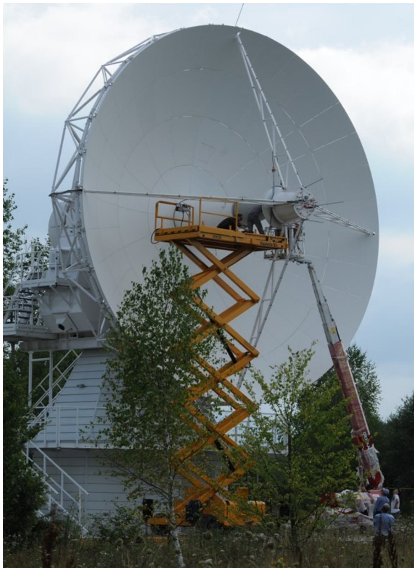
Fig.1 RT-13 noise temperature measurements by using wide aperture low temperature noise generator
