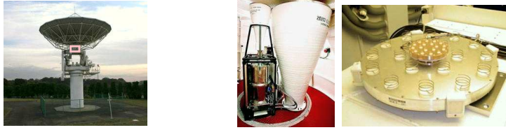
Figure 90: In order to make the reference point visible from outside, one usually has to place whole feed and receiver system in a small cabin in the back structure of the main reflector (Left). For that purpose, we need compact feed systems. Examples of compact feeds, 1.4 GHz/2.3 GHz feed horn used in Australian Telescope, and helical array S/X feed used in VERA, are shown in right two panels.
