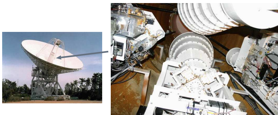
Figure 88: Feed horns and receivers of 34 m VLBI antenna (Left) at Kashima, Japan, for various frequency bands are uplifted to the focus one by one, along rails inside the “Feed Cone” (Right).
