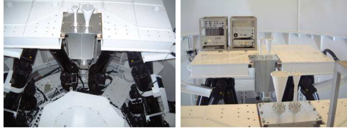
Figure 103: He-cooled 22 GHz and 43 GHz HEMT amplifiers placed in common cryogenic dewars and mounted on VERA dual-beam receiving system.
