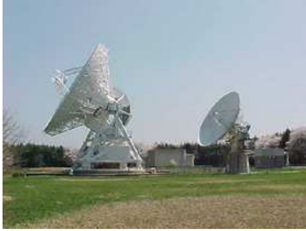
Figure 8: Wheel & Track (left) and Yoke & Tower (Right) antennas.
