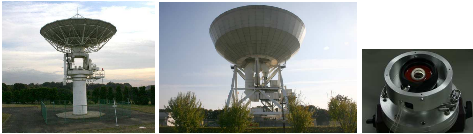
Figure 11: 11 m antenna at Kashima, Japan, with the reference point directly visible from outside (Left), and 32 m antenna at Tsukuba, Japan, with the reference point invisible from outside (Middle). Also shown is a cat's eye used in ground geodetic measurements.
